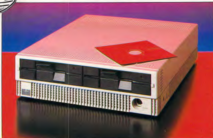
The two, half-height disk drives occupy most of the front panel
